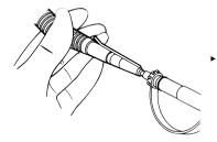
Remove the cutter or grinder, place the spray nipple tip in the opening and spray.
