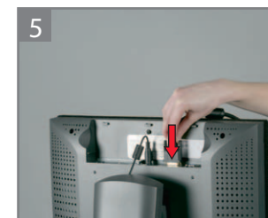
5 Connect the HDMI cable to a suitable monitor or screen.
