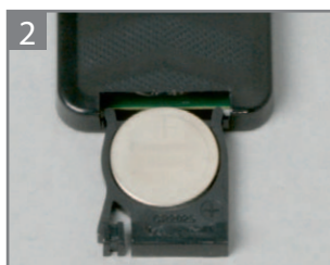
Replace the battery. (Button battery type CR2032)
