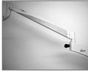
Move the swing arm upwards. Light switches off automatically.
