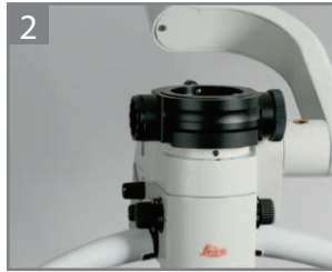
2 Fit the beam splitter. For 50/50 % or 70/30 % observation.
